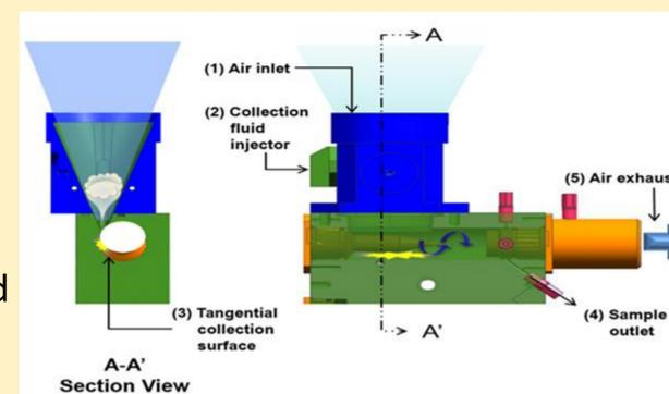
Figure 3. Wetted Wall Cyclone used for aerosol collection
